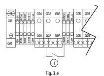
Contact open: humiFog deactivated Contact closed: humiFog activated
