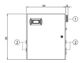
detail of cabinet, air & water inlet side view
